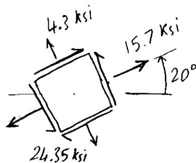
7. A close-ended cylinder of internal radius of  $r_i = 30$  in and a wall thickness of  $t = 1$  in. The pressure inside the cylinder is  $P_i = 8$  psi. The cylinder is also subjected to torque of  $T = 500$  lb.in applied at both ends. Find the state of stress at a point on the surface of the cylinder and show it on a stress element.
