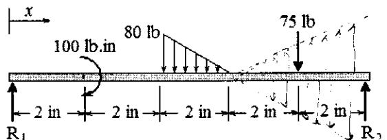
$$q(x) = R_1 \langle x \rangle^1 - 100 \langle x-2 \rangle^2 - 80 \langle x-4 \rangle^0 + \frac{80}{2} \langle x-4 \rangle^1 + \frac{80}{2} \langle x-6 \rangle^1 - 75 \langle x-8 \rangle^1 + R_2 \langle x-10 \rangle^1$$
