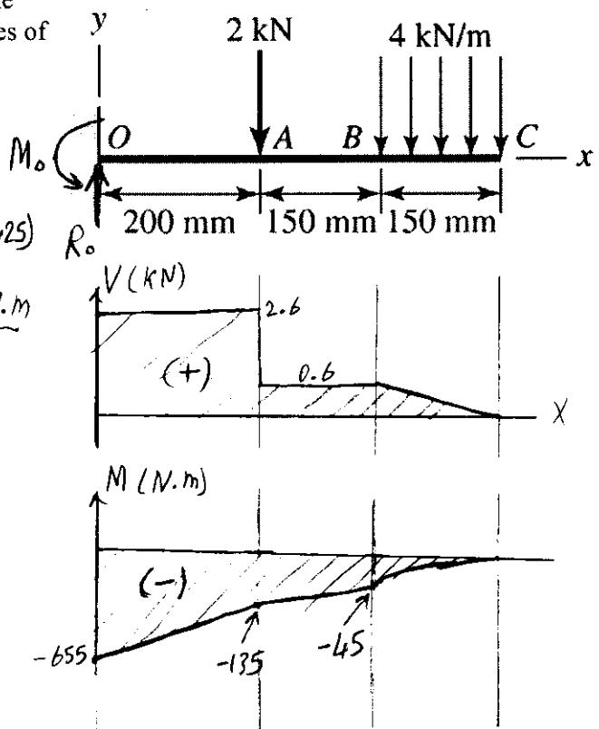
3. Using singularity functions derive the expressions for the loading, shear force, and bending moment for the beam shown.
