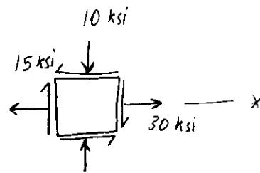
6. If the state of stress at a point is given as  $\sigma_x = 30 \text{ ksi}$ ,  $\sigma_y = -10 \text{ ksi}$ ,  $\tau_{xy} = -15 \text{ ksi}$ , using Mohr's circle find:
