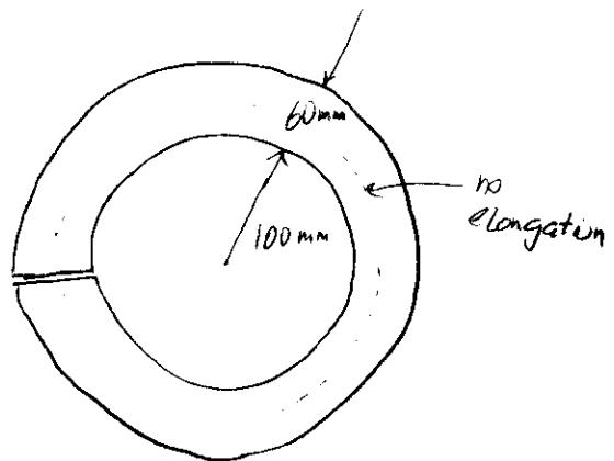
From Table A-22, the fracture strain for AL 7075-T6 :  $\epsilon_f = 0.18$
