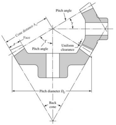
Standard straight-tooth bevel gears are cut using 20° pressure angle.
