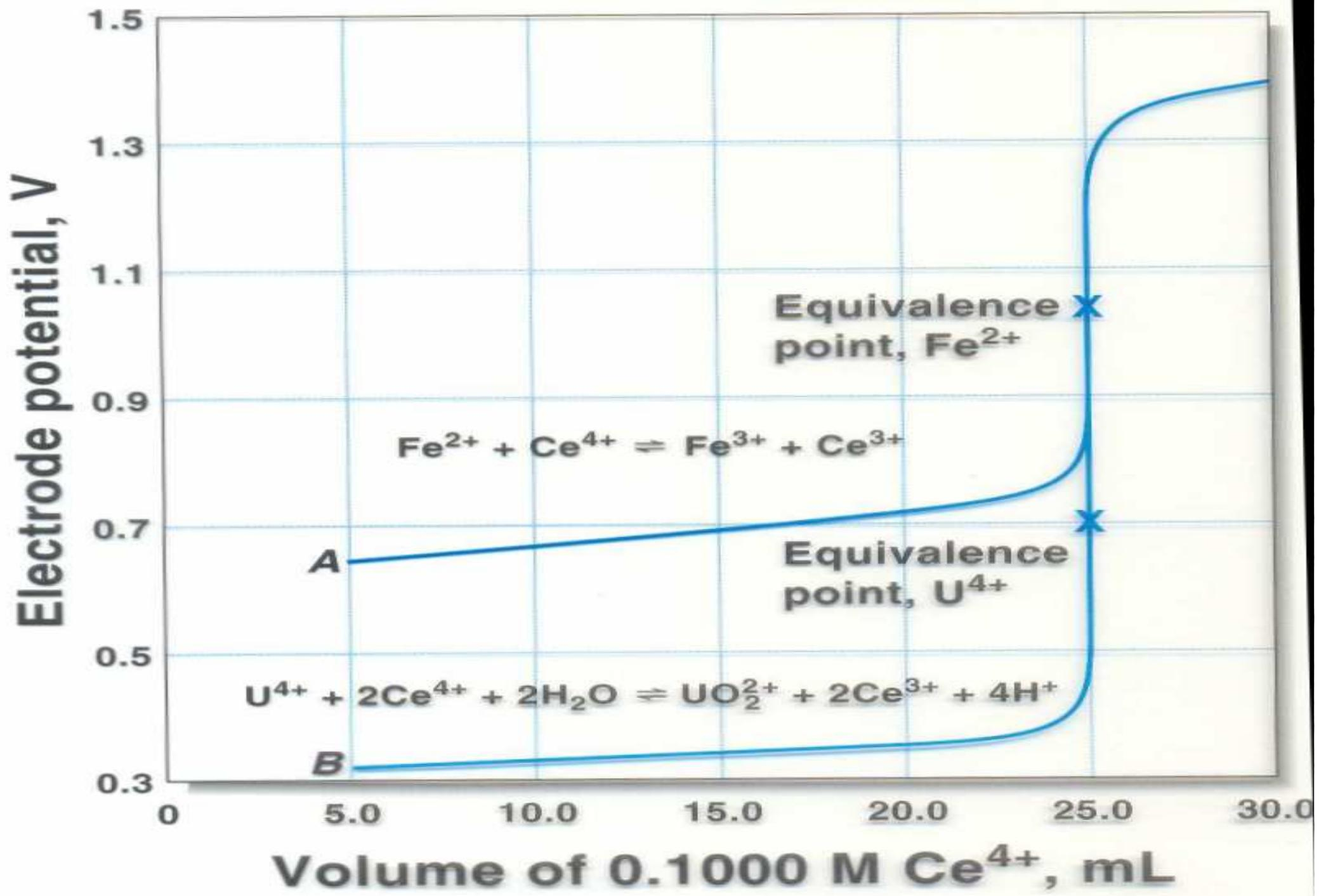
Consider the titration of 50.00 mL of 0.0500 M  $\text{Fe}^{2+}$  with 0.1000 M  $\text{Ce}^{4+}$  in a medium that is 1.0 M in  $\text{H}_2\text{SO}_4$  at all times. Formal potential data for both half-cell processes are available in Appendix 4 and are used for these calculations. That is,
