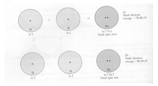
Figure 57: The effect of Pauli principle on the repulsive energy between two hydrogen atoms.
