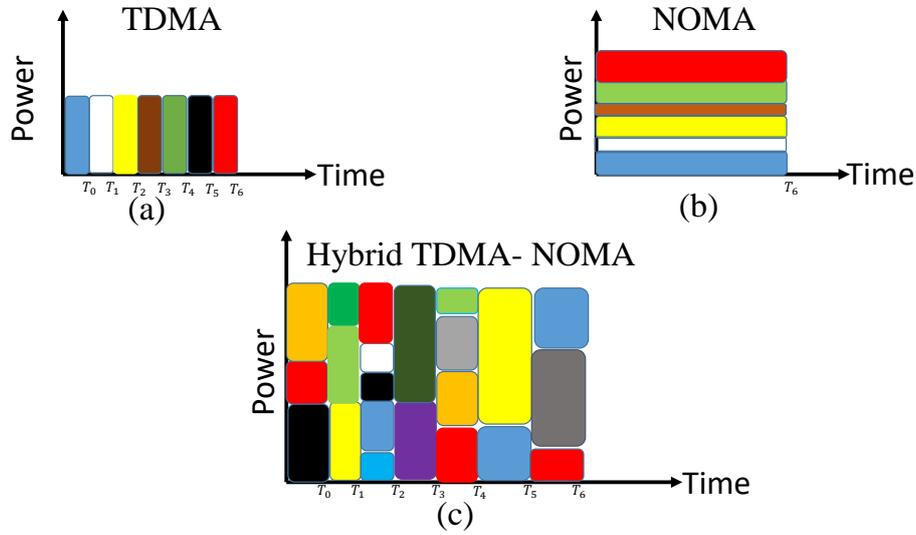
Fig. 2.4 An illustration of different MA approaches: (a) TDMA approach, (b) NOMA approach, (c) Hybrid TDMA-NOMA approach.
