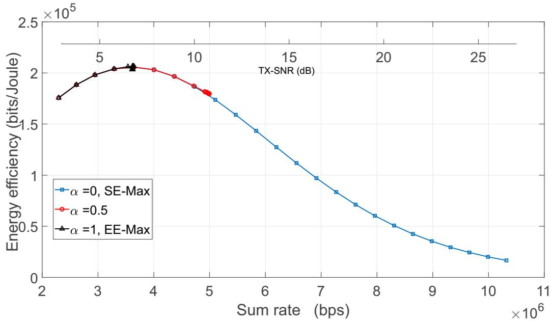
Fig. 5.1 Achieved EE and sum rate against TX-SNR with different weight factors  $\alpha$ .
