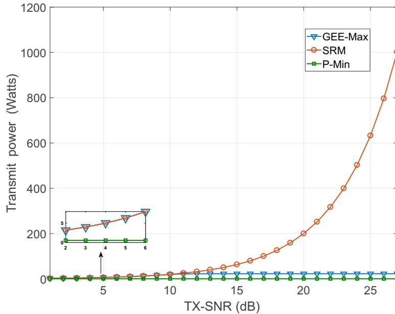
Fig. 4.6 Required transmit power for different beamforming design criteria.
