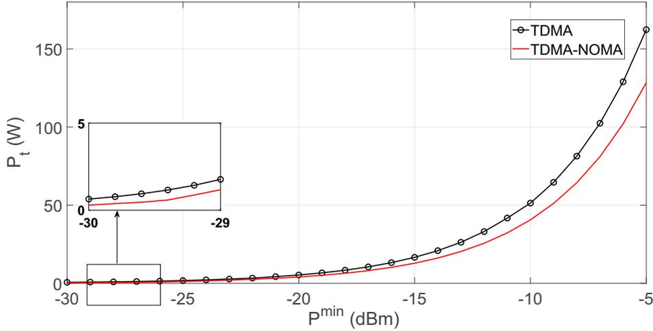
Fig. 6.3 The required transmit power versus different minimum harvest power requirements  $P^{\min}$ , with a minimum rate requirement  $R^{\min} = 10^{-1}$  bit/Hz.
