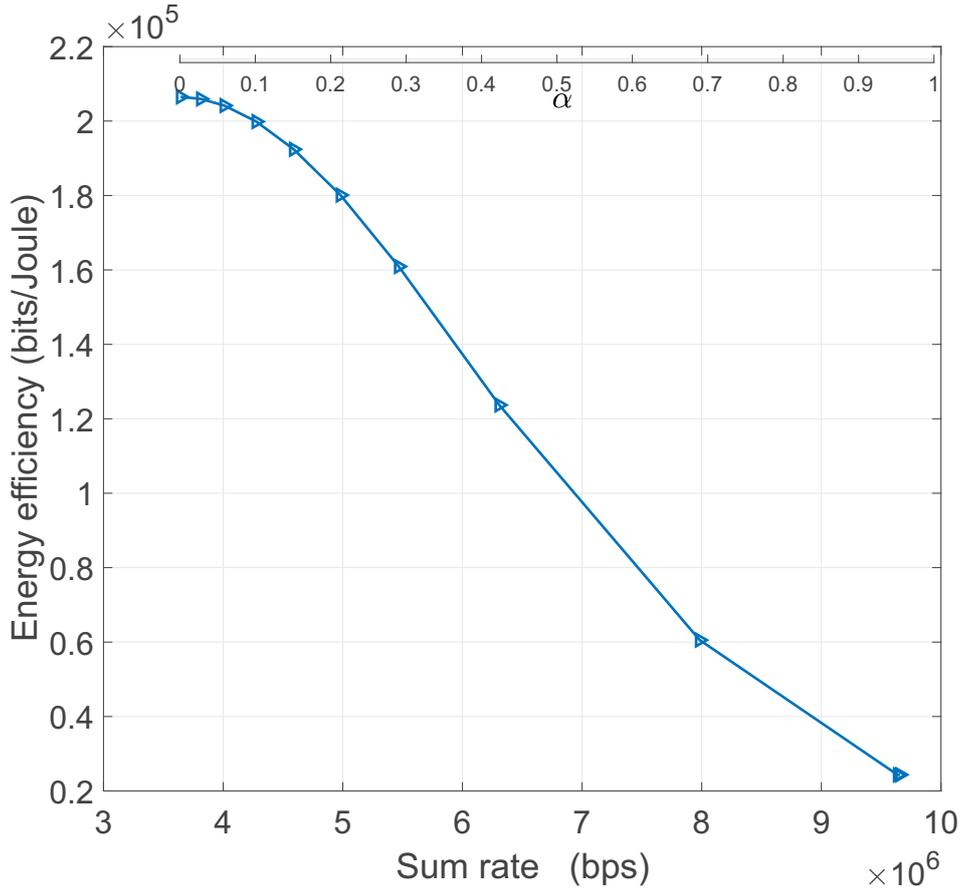
Fig. 5.5 Pareto front of SE-EE trade-off-based design for TX-SNR = 24 dB.
