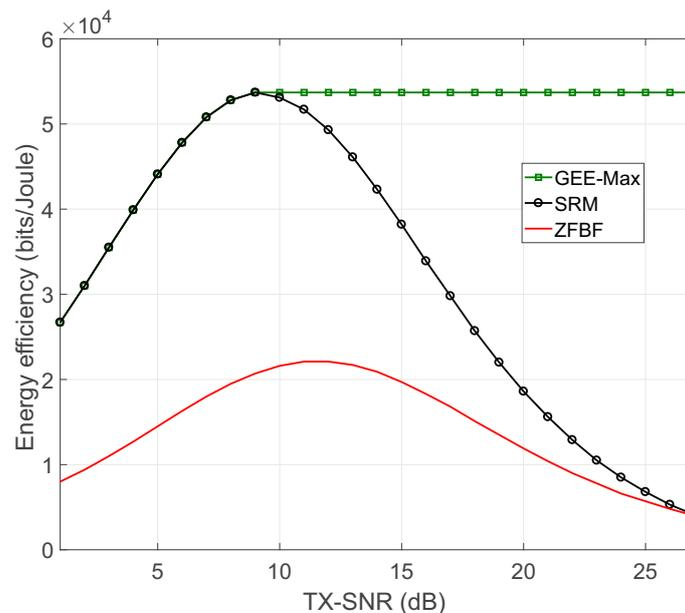
Fig. 4.3 EE for different design criteria.
