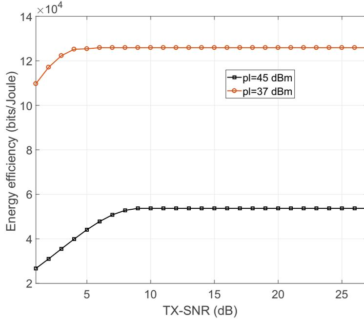
Fig. 4.7 Achieved EE of GEE-Max design with different power losses.
