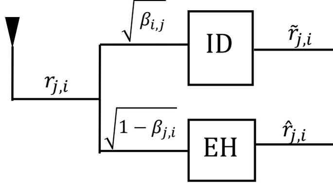
Fig. 6.2 Illustration of splitting the received signal at  $u_{j,i}$ .
