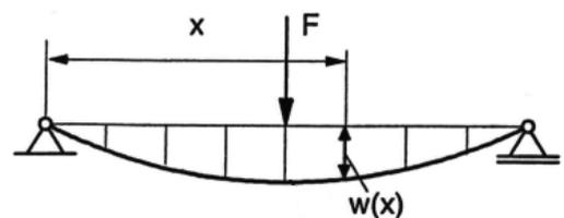
Figure 2: Bar on two supports.
