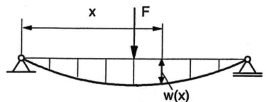
Figure 2: Bar on two supports.
