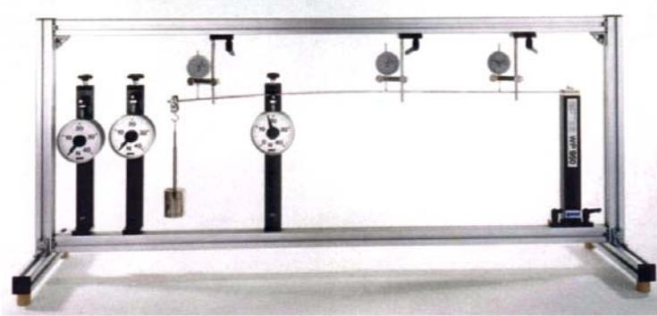
**Procedure:****Part 1:****Measurement of the reaction forces:**
