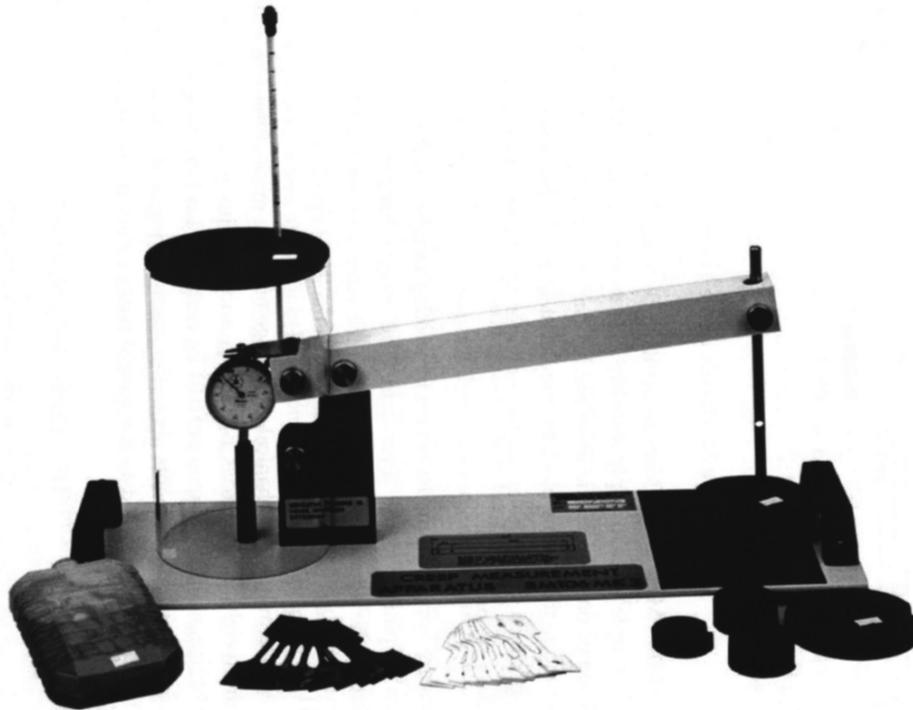
Figure 2 Components of the SM106 Mk II Apparatus
