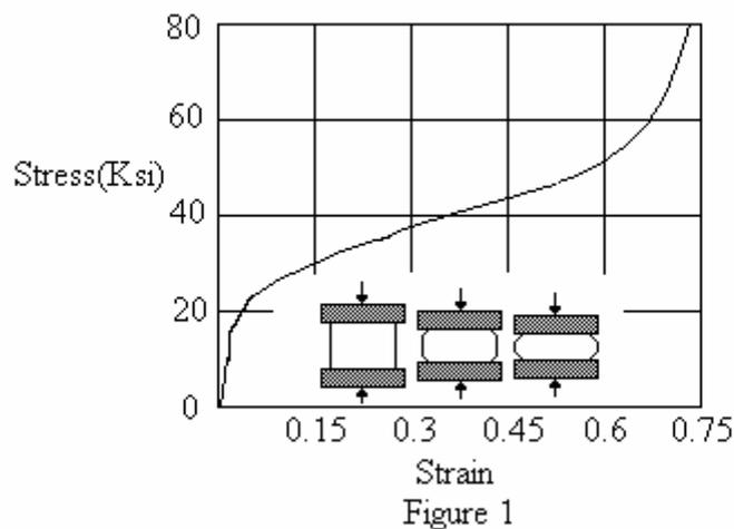
Brittle materials in compression typically have an initial linear region followed by a region in which the shortening increases at a higher rate than does the load. Thus, the compression stress-strain diagram has a shape that is similar to the shape of the tensile diagram. However, brittle materials usually reach much higher ultimate stresses in compression than in tension. Also, unlike ductile materials in compression, brittle materials actually fracture or break at the maximum load.
