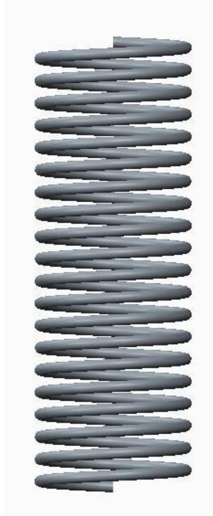
Helical Sweep : Helical Path and Section
