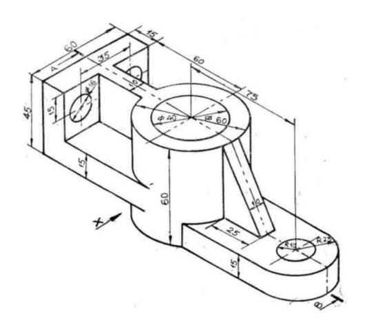
**Problem Two**: (8 Points) Using **Mirror & Pattern CREO Commands**, create a CREO solid model of the part shown below.
