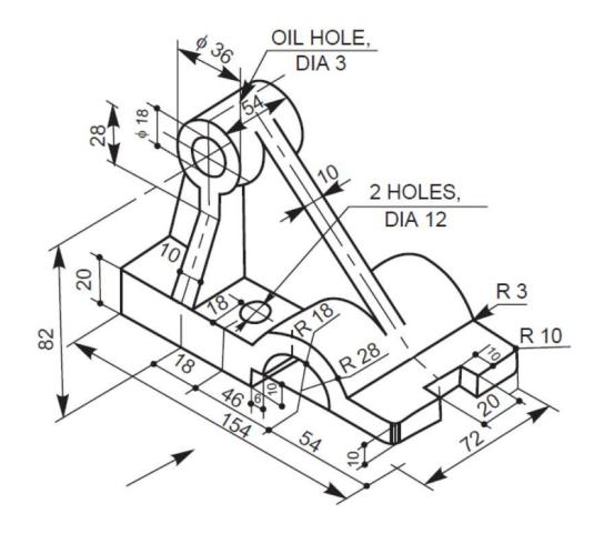
**Problem Two:** (10 Points) Using CREO Parametric <u>Blend</u> Command, draw the following 3D part and save it as ProblemTwo.prt.
