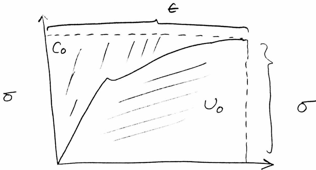
$U_0$  is the strain energy density = area under Curve
