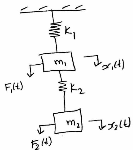
$$\{F(t)\} = \begin{Bmatrix} F_1(t) \\ F_2(t) \end{Bmatrix} \quad F_1(t) = F_1 \cos \omega t \\ F_2(t) = F_2 \cos \omega t$$
