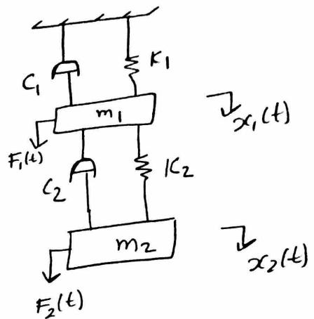
In All cases above, If we want to find natural Frequencies and modeshapes, we drop (or remove) any damping and forcing terms so the equation of motion would become:-
