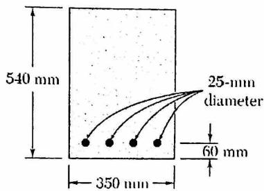
**PROBLEM 4.47** The reinforced concrete beam shown is subjected to a positive bending moment of 175 kN · m. Knowing that the modulus of elasticity is 25 GPa for the concrete and 200 GPa for the steel, determine (a) the stress in the steel, (b) the maximum stress in the concrete.
