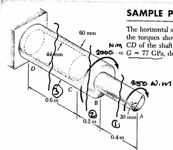
The horizontal shaft  $AD$  is attached to a fixed base at  $D$  and is subjected to the torques shown. A 44-mm-diameter hole has been drilled into portion  $CD$  of the shaft. Knowing that the entire shaft is made of steel for which  $G = 77 \text{ GPa}$ , determine the angle of twist at end  $A$ .
