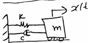
In this system, we need only one variable to describe the motion of the system ( $x(t)$ )
