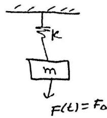
$$x(t) = \left(x_0 - \frac{F_0}{w_n^2}\right) \cos w_n t + \frac{v_0}{w_n} \sin w_n t + \frac{F_0}{w_n^2}$$
