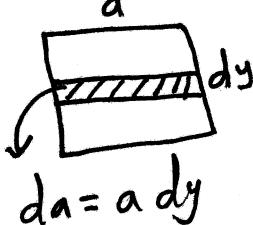
$$\begin{aligned} \Phi &= \int \vec{B} \cdot d\vec{a} = \int_B da = \int_0^a B a dy \\ &= kt^2 a \int_0^a y^3 dy \\ &= \frac{1}{4} kt^2 a^5 \text{ as expected.} \end{aligned}$$
