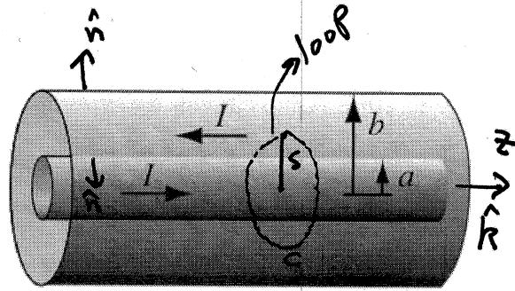
**Problem 6.17** A current  $I$  flows down a long straight wire of radius  $a$ . If the wire is made of linear material (copper, say, or aluminum) with susceptibility  $\chi_m$ , and the current is distributed uniformly, what is the magnetic field a distance  $s$  from the axis? Find all the bound currents. What is the net bound current flowing down the wire?
