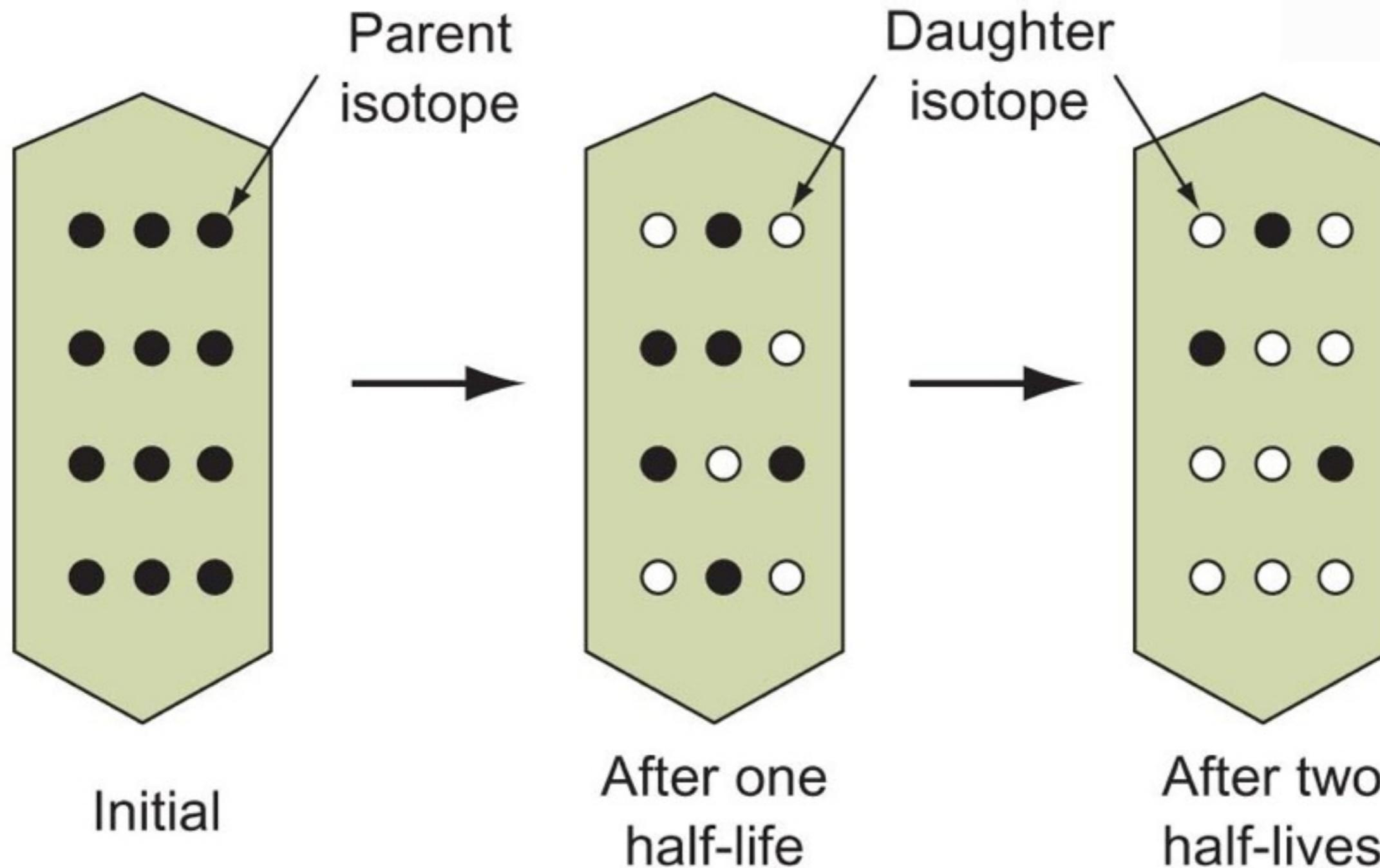
Schematic diagram showing decay of radioactive *parent* isotope (e.g. U-238) to a *daughter* (e.g. Pb-206). The original isotope was sealed in a mineral grain at time of crystallization. Note changing ratio of parent/daughter after 2 half-lives. Note that to get an estimate of the geologic age, you need the ratio of the parent isotope to the daughter isotope, e.g. two measurements.
