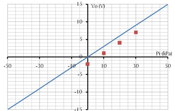
If the same instrument was used to measure pressure values of ( 0,10 , 20 ,and 30 kPa ) at a different location and gave the results shown in figure ( square markers ). The error shown represents :
