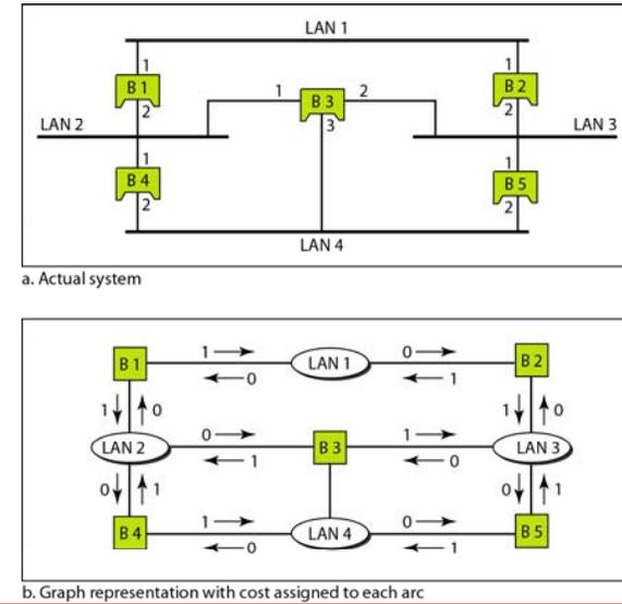
**Figure 15.9** Finding the shortest paths and the spanning tree in a system of bridges
