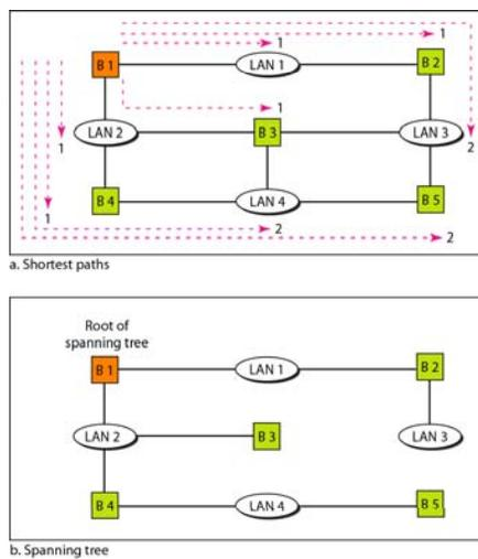
**Figure 15.10** Forwarding and blocking ports after using spanning tree algorithm
