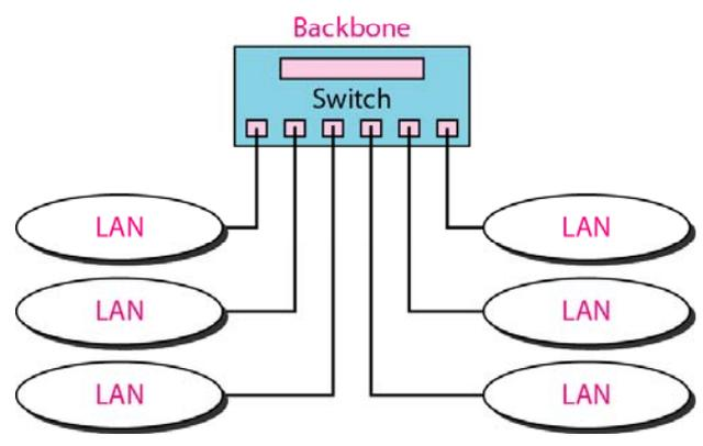
**Figure 15.14** *Connecting remote LANs with bridges*
