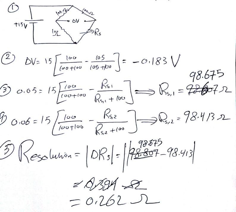
A wheatstone Bridge with  $R1 = R2 = R3 = 100 \Omega$ . The sensor (R4 = Rs) has a nominal resistance of 100  $\Omega$ . Vs = 10 V.
