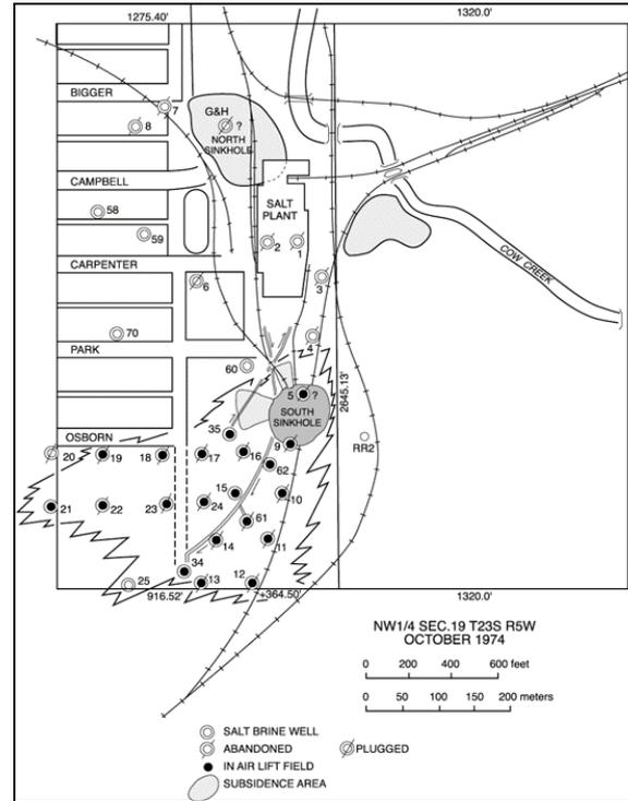
Cargill Plant Layout, Showing North and South Sinkholes
