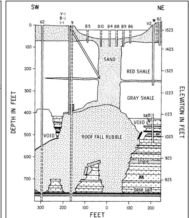
Cross Section Through South Sinkhole, Cargill Site
