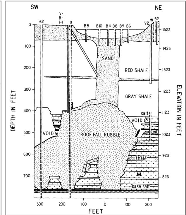
Cross Section Through South Sinkhole, Cargill Site
