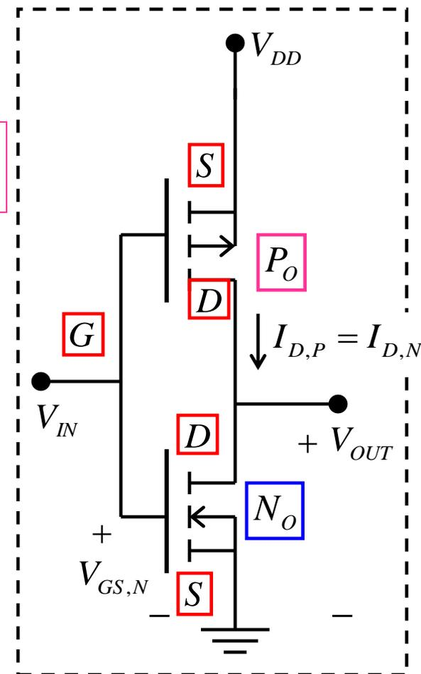
Invalid since  $V_{SD}$  has to be less than  $(V_{SG} + V_{TP})$
