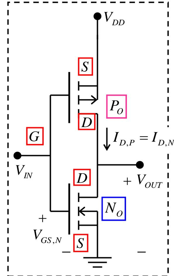
Invalid since  $V_{DS}$  has to be less than  $(V_{GS} - V_{TN})$
