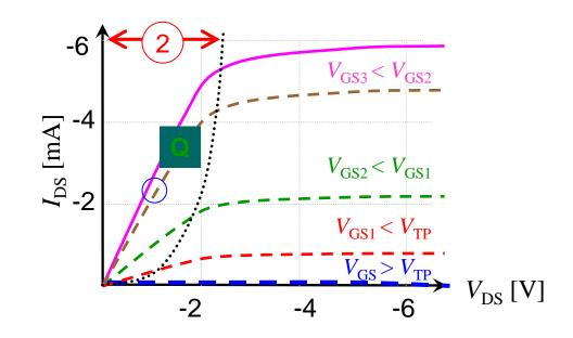
$$I_{SD} = \frac{K_p}{2} \left[ 2 \times (V_{GS} - V_{TP}) V_{DS} - V_{DS}^2 \right]$$
