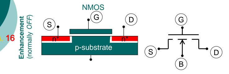
The Drain-to-Source current (electrons are emitted from the source to the drain)  $I_{\text{DS}} > 0$
