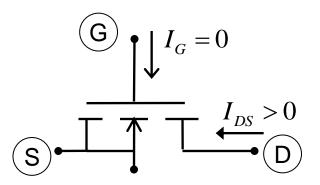
$$I_{DS} = \frac{K_n}{2} (V_{GS} - V_{TN})^2$$
