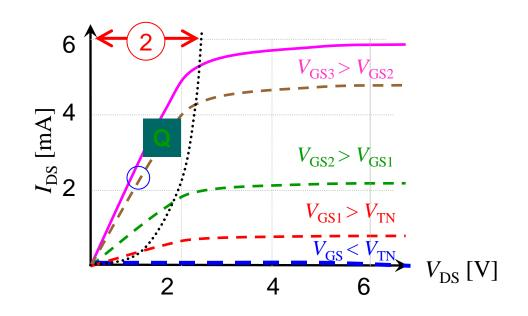
$$I_{DS} = \frac{K_n}{2} \left[ 2 \times (V_{GS} - V_{TN}) V_{DS} - V_{DS}^2 \right]$$
