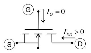
$$I_{SD} = \frac{K_P}{2} (V_{GS} - V_{TP})^2$$
