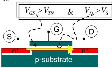
V<sub>TN</sub> is the threshold voltage and defined as the minimum V<sub>GS</sub> needed to create a channel between the source and the drain
