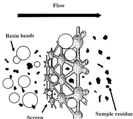
Fig. 3. Depiction of the screen at the end of the mini-column for retention of analyte on anion exchange resin beads and passage of the insoluble sample residue to waste.
