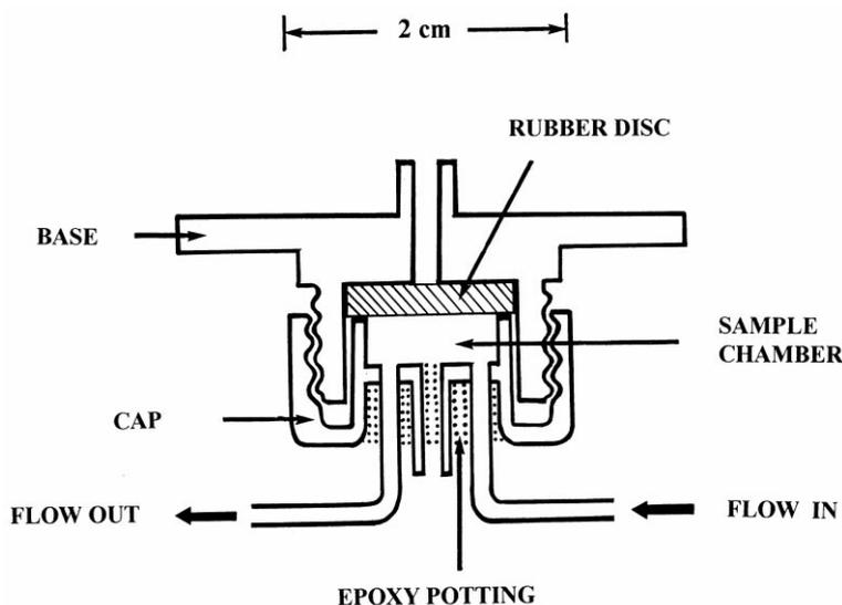
Fig. 2. A cross-section of the solid sample insertion chamber. The material of construction is PVC and Teflon, and the nominal chamber volume is  $0.25 \text{ cm}^3$ .
