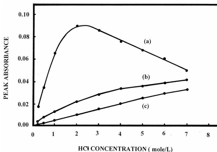
Fig. 4. The effect of HCl concentration on the retention of the chloro-complexes of  $\text{Zn}^{2+}$  (a),  $\text{Cu}^{2+}$  (b) and  $\text{Fe}^{3+}$  (c) as detected by atomic absorption spectrometry after elution with 0.1 M  $\text{HNO}_3$  solution.
