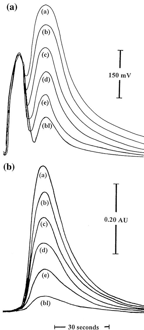
Fig. 5. Calibration signal profiles for the determination of iron in multi-vitamin tablets by on line solid sample digestion and flow injection analysis with spectrophotometric (a) and atomic absorption (b) detection. (a) 500  $\mu\text{g}$ ; (b) 400  $\mu\text{g}$ ; (c) 300  $\mu\text{g}$ ; (d) 200  $\mu\text{g}$ ; (e) 100  $\mu\text{g}$ ; (bl) blank.
