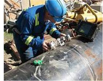
In general, ultrasonic testing is based on the capture and quantification of either the reflected waves (*pulse-echo*) or the transmitted waves (*through-transmission*). Each of the two types is used in certain applications, but generally, pulse echo systems are more useful since they require one-sided access to the object being inspected.
