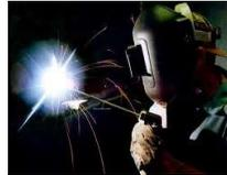
The most commonly used welding process is **Arc Welding** where a power supply is used to create and maintain an electric arc between an electrode and the base material to melt metals at the welding point
