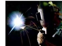
The most commonly used welding process is **Arc Welding** where a power supply is used to create and maintain an electric arc between an electrode and the base material to melt metals at the welding point
