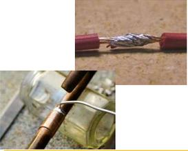
Soldering differs from welding in that soldering does not involve melting the work pieces
