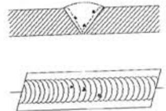
*Oxide Inclusions*: This type of inclusions results from the presence of high melting point oxides on the base metal which mixes with the molten material during welding.
