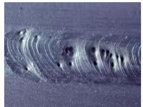
clustered together (*cluster porosity*). In general, porosity can result from the presence of dirt, rust or moisture on the surface of base or filler metal. Also, it could result from high sulfur content in the base metal or excessive arc length.
