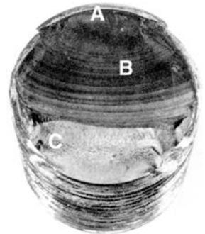
The presence of the crack can (and should) be detected during the crack growth stage (stage 2) before the component suddenly fails.
