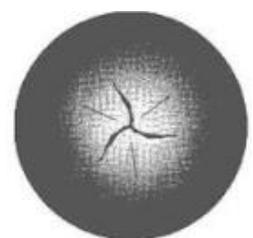
cracks and tears will develop because the surrounding material has already solidified.
