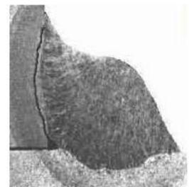
the weld metal during cooling or after a period of time (hours or even days). The sources of hydrogen which leads to this type of cracks may include moisture in the electrode shielding, the shielding gas or base metal surface, or contamination of the base metal with hydrocarbon (oil or grease).
