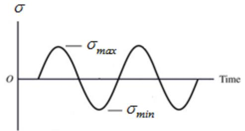
In the case of the rotating shaft subjected to both radial and axial loads (such as with helical gears) the fluctuating stress pattern will be different since there will be a component of stress that is always present (*due to the axial load*).
