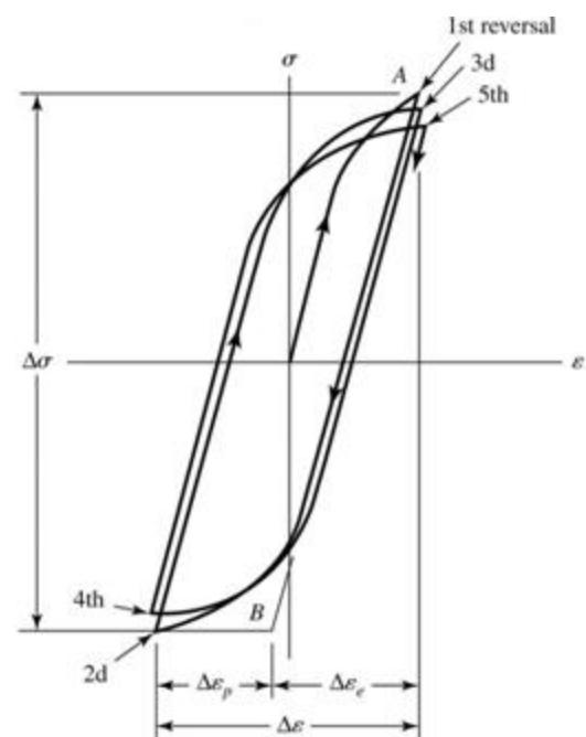
means that the material has been softened in the reverse loading direction (*this is referred to as Bauschinger Effect*). Each time the stress is reversed, the yield strength in the other direction is decreased and the material gets softer and undergoes more plastic deformation until fracture occurs.
