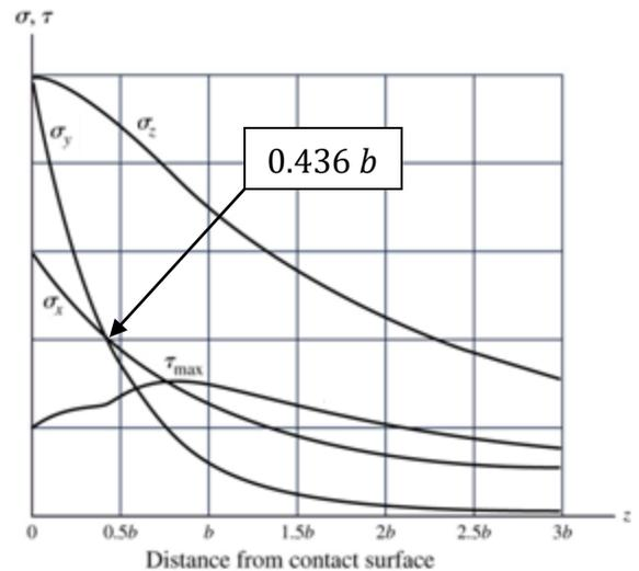
Hertz equations are valid if the contact surface is free of shear stress ( $F$  only).
