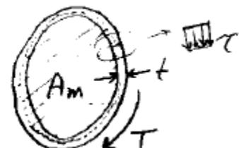
For closed thin-walled tubes (of any shape) the shear stress is assumed to be constant through-out thickness.
