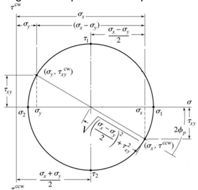
measured from the  $x$  direction, is found by determining the angle  $2\phi_p$  from the circle and rotating in the same direction.
