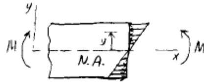
Where,  $y$ : is the height from the neutral axis (centroidal axis)
