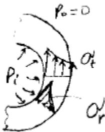
$$\sigma_t = \frac{P_i r_i^2}{r_o^2 - r_i^2} \left( 1 + \frac{r_o^2}{r^2} \right)$$
