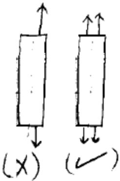
$$\sigma = \frac{F}{A} \quad \begin{cases} (+) \text{ For Tension} \\ (-) \text{ For compression} \end{cases}$$
