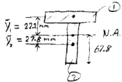
$$I = I_1 + I_2 = (\bar{I}_1 + A_1 \bar{y}_1^2) + (\bar{I}_2 + A_2 \bar{y}_2^2)$$
