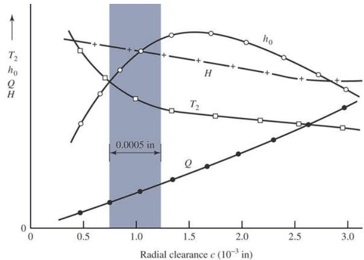
film thickness “ $h_0$ ” increases with clearance then it starts to decrease.
