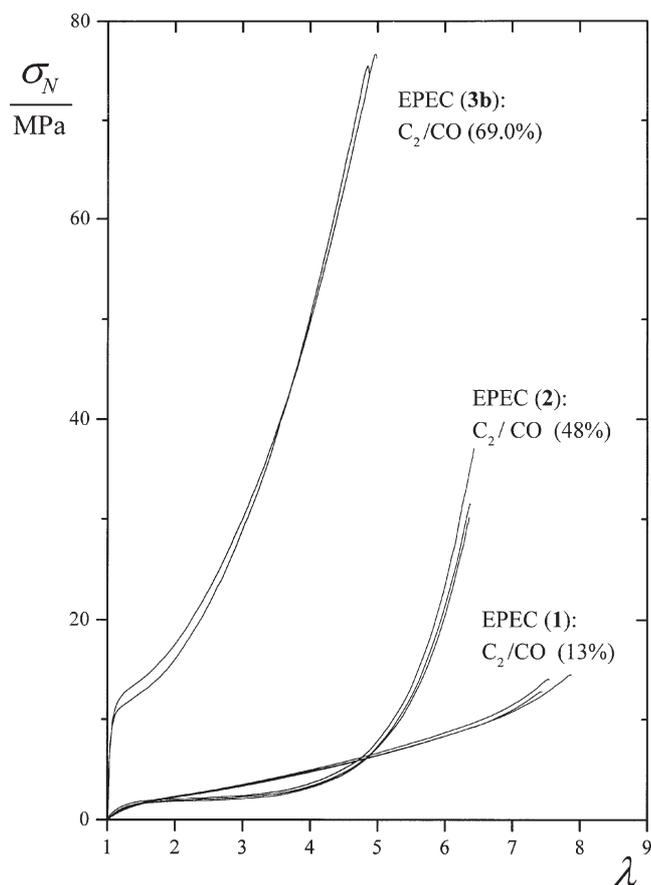
Figure 7. Stress-strain properties of high molecular weight propene-ethene-CO terpolymers (EPEC **1**, E-CO = 13 mol%,  $M_w = 5.9 \times 10^5$  g/mol; EPEC **2**, E-CO = 48 mol%,  $M_w = 4.1 \times 10^5$  g/mol; EPEC **3b**, E-CO = 69 mol%,  $M_w = 12.0 \times 10^5$  g/mol).
