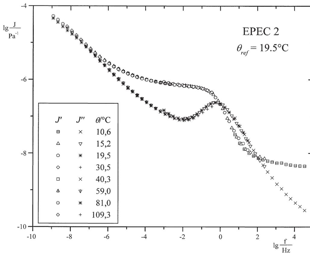
Figure 9. Mastercurve of the terpolymer EPEC 2.
