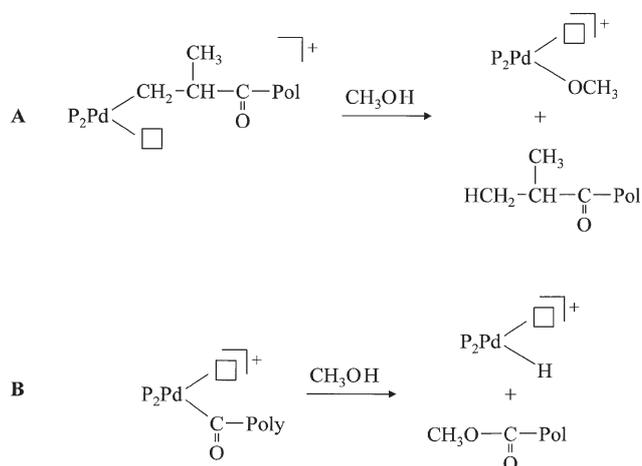
Figure 4. Methanol as chain termination agent.
