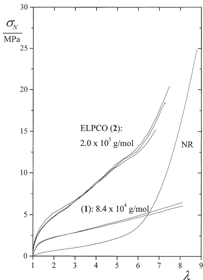
Figure 6. Stress-strain behavior of propene-CO copolymers (1,  $M_w = 8.4 \times 10^4$  g/mol; 2 (ELPCO)  $M_w = 2.0 \times 10^5$  g/mol) and of a polyisoprene (NR) ( $\sigma_n$ , nominal stress;  $\lambda$ , extension ratio).
