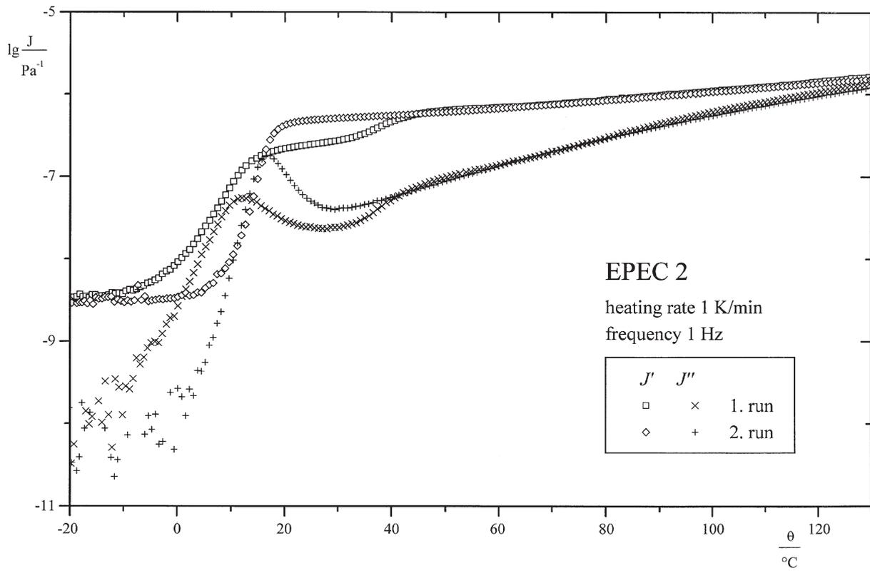
Figure 8. Shear compliance of the terpolymer EPEC 2 during two temperature runs.
