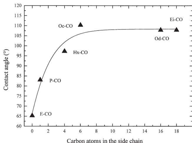
Figure 14. Sessile drop contact angles of water drops on films of a series of copolymers (ethene/CO (E-CO), propene/CO (P-CO), hexene/CO (Hx-CO), octene/CO (Oc-CO), octadecene/CO (Od-CO), icosene/CO (Ic-CO)).
