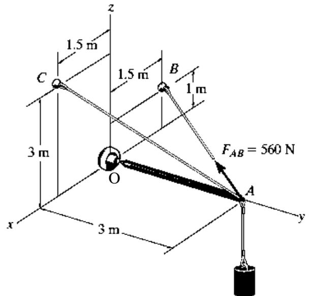
**Q.3 (5 points)** Determine the resultant force and resultant moment at point O. Express the results as Cartesian vectors. What is the magnitude and direction of the resultant moment at O.
