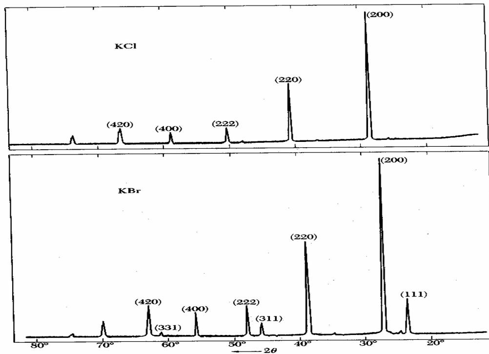
Figure 40: The x-ray diffraction from KCl and KBr powders.
