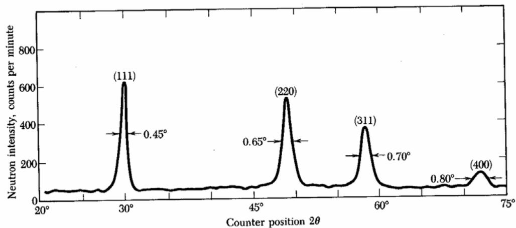
Figure 41: Neutron diffraction pattern for powdered diamond.
