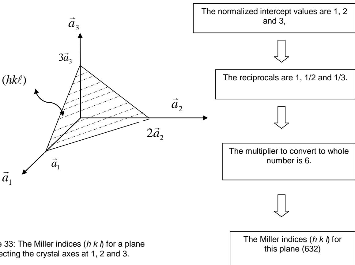
Figure 33: The Miller indices ( $h k l$ ) for a plane intersecting the crystal axes at 1, 2 and 3.
