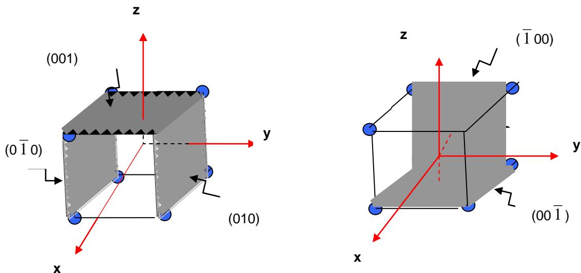
Figure 35: A family of lattice planes in a simple cubic lattice
