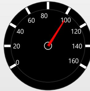
Speedometer reads magnitude of velocity (speed)  $100 \text{ km/h}$
