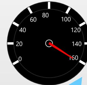
Speedometer reads magnitude of velocity (speed)  $160 \text{ km/h}$
