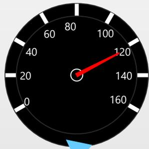
Speedometer reads magnitude of velocity (speed)  $120 \text{ km/h}$
