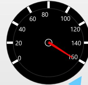
Speedometer reads magnitude of velocity (speed) 160 *km/h*
