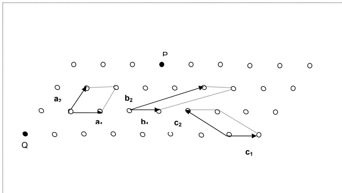
**Figure 2:** Three different choices of pairs of primitive vectors. Each set gives the smallest possible parallelogram area.
