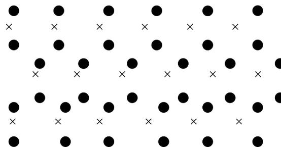
Figure 1: Periodic crystal structure is described as a lattice with basis
