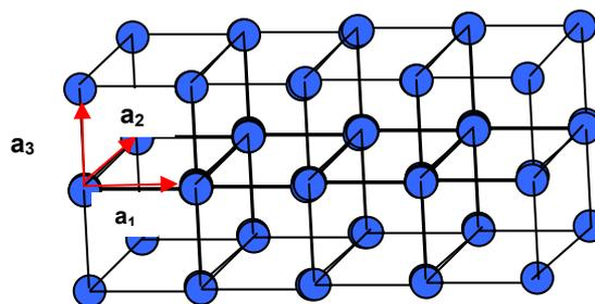
Figure 3: Three dimensional primitive cell is shown in a periodic crystal structure.
