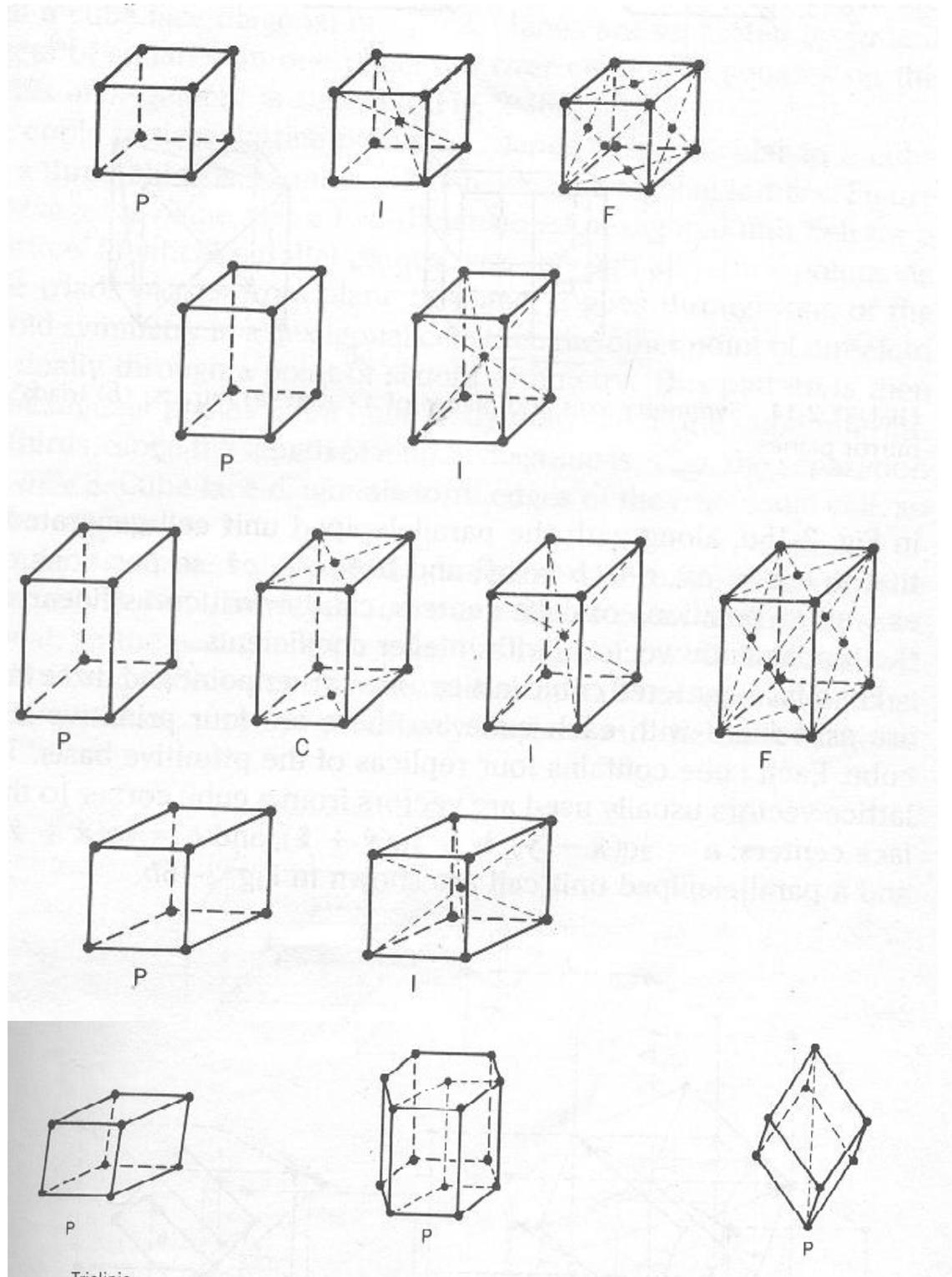
Figure 53: The 7 crystal systems divided into 14 Bravais lattices
