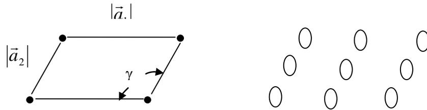
Figure 48: Oblique unit cell with its symmetry elements
