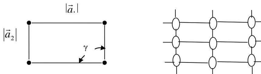
Figure 49: Rectangular unit cell with its symmetry elements
