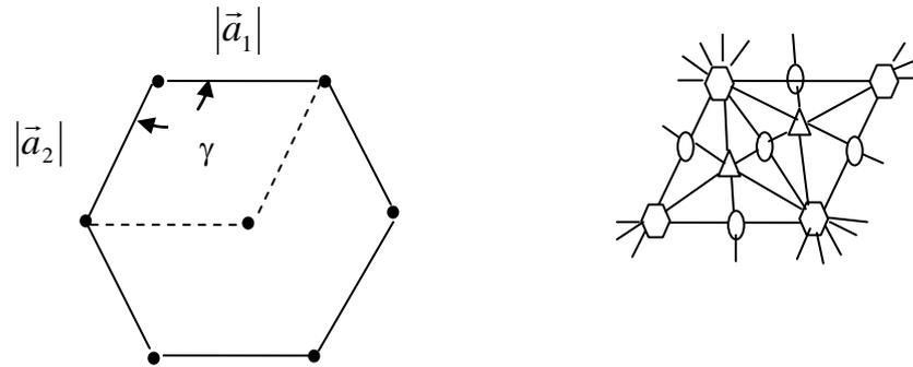
Figure 52: Hexagonal unit cell with its symmetry elements
