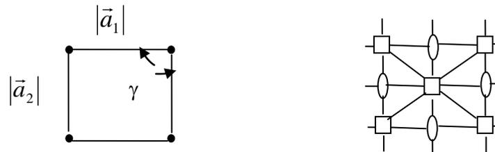
Figure 51: Square unit cell with its symmetry elements
