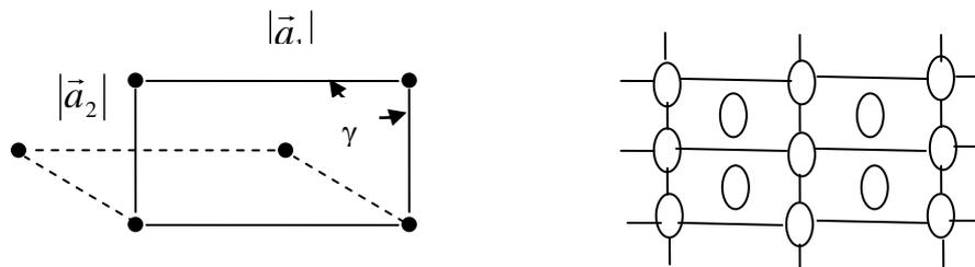
Figure 50: Centered rectangular unit cell with its symmetry elements
