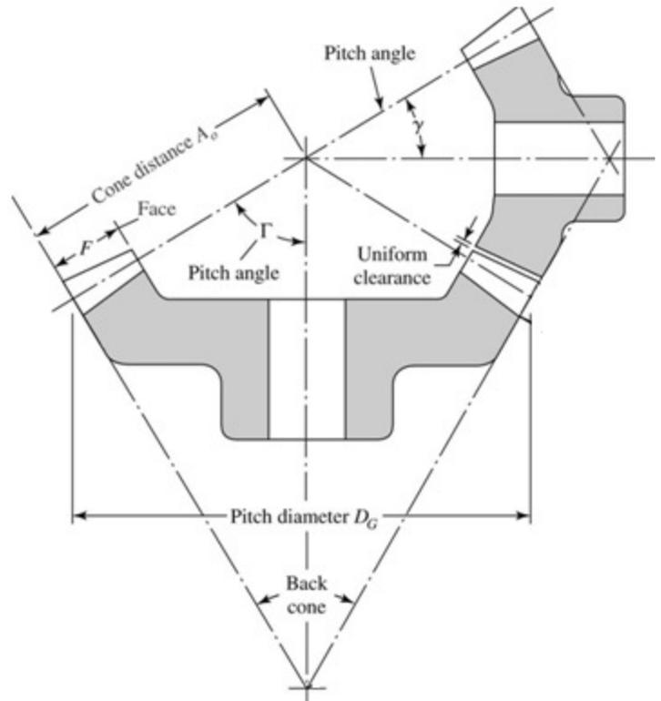
Standard straight-tooth bevel gears are cut using  $20^\circ$  pressure angle.
