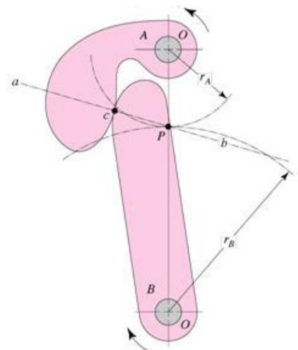
The angular-velocity ratio is inversely proportional to the ratio of radii of the pitch circles of mating gear.
